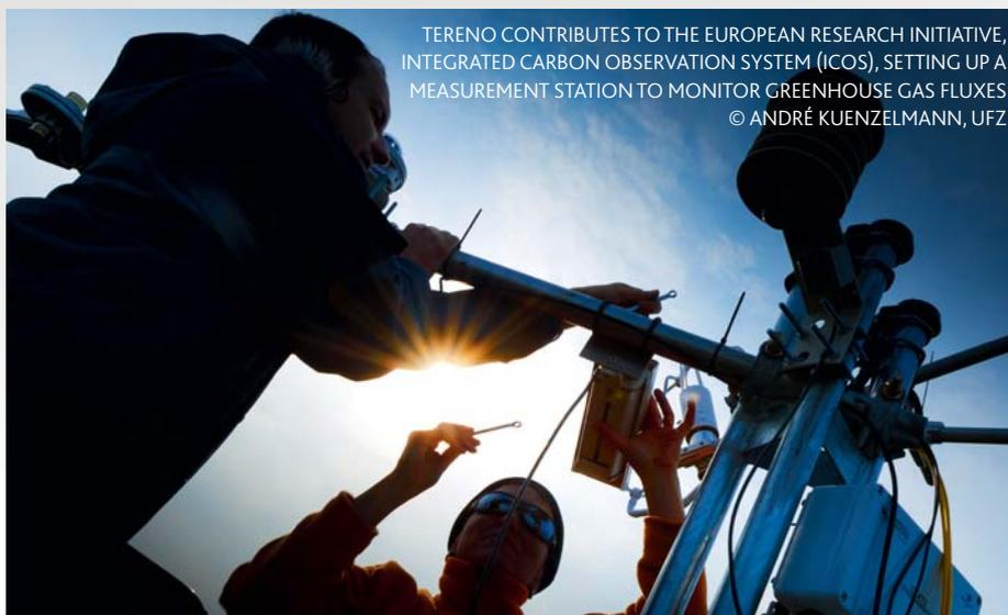
TERENO CONTRIBUTES TO THE EUROPEAN RESEARCH INITIATIVE, INTEGRATED CARBON OBSERVATION SYSTEM (ICOS), SETTING UP A MEASUREMENT STATION TO MONITOR GREENHOUSE GAS FLUXES
