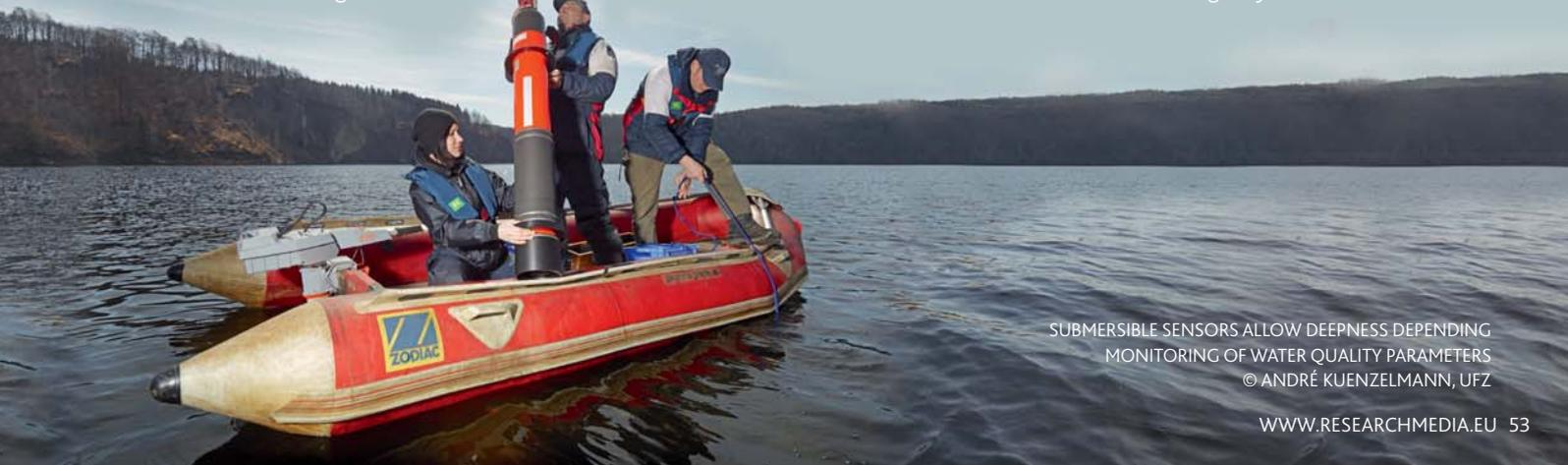
SUBMERSIBLE SENSORS ALLOW DEEPNESS DEPENDENT MONITORING OF WATER QUALITY PARAMETERS
