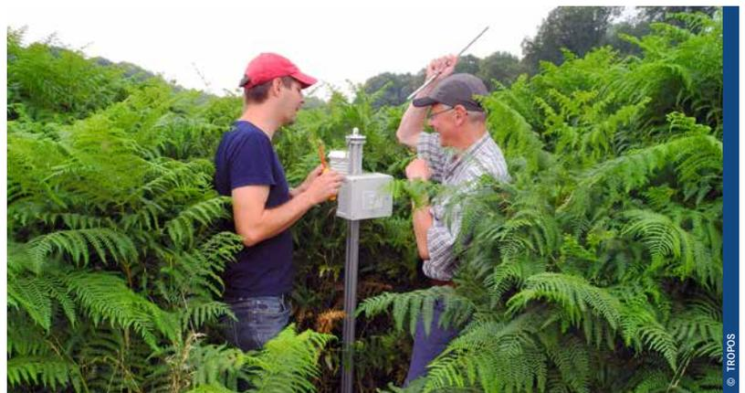
*Near Jülich, TROPOS scientists installed roughly 100 pyranometers, which collect data on solar radiation levels.*
