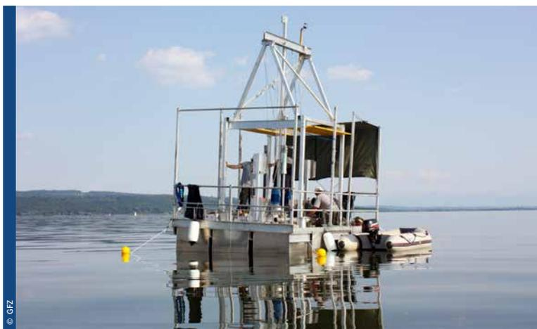
Researchers gather sediment profiles from the bottom of Lake Ammersee with the help of a drilling platform.
