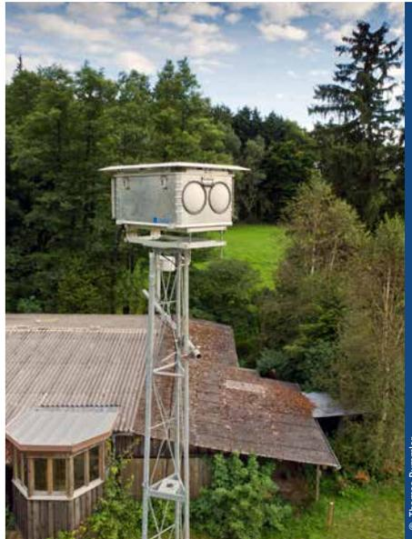
*The Fendt test site in the "Bavarian Alps/pre-Alps" TERENO observatory features a newly developed microwave measurement system, which can monitor air moisture and precipitation near the surface.*
