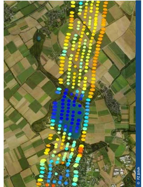
*Radiometers provide precise data on soil moisture, but with low spatial resolution. Here, measurements are taken on a flight above the Blausteinsee lake near Jülich.*
