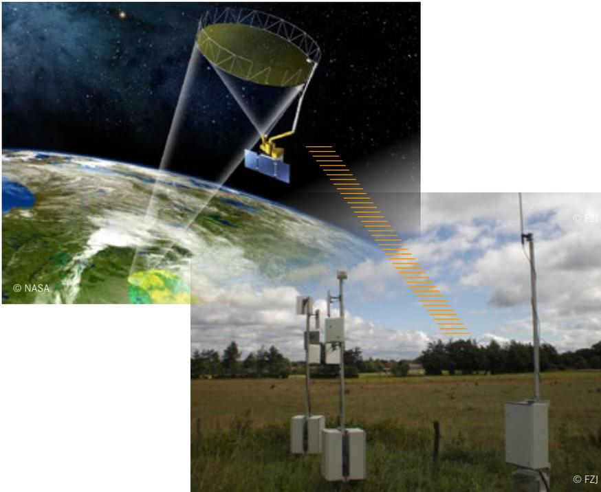
With the help of SMAP satellite data, researchers can generate very precise estimates of soil moisture content. Satellite data is compared with ground-based measurements taken at stations such as TERENO’s Rollesbroich site.
