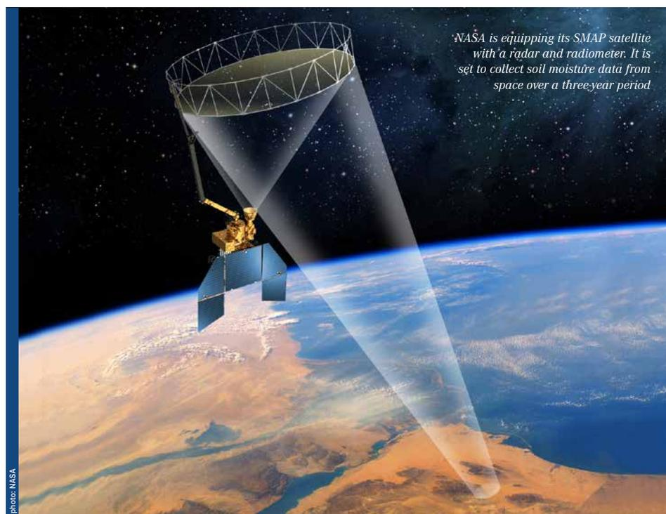
*NASA is equipping its SMAP satellite with a radar and radiometer. It is set to collect soil moisture data from space over a three-year period*
