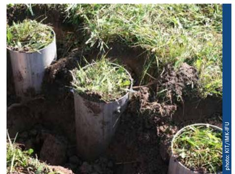
*Climate simulation with small lysimeters*
