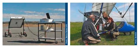
Successful testing: Researchers from the UFZ are able to measure soil moisture with a PLMR sensor (left) by combining their recordings with vegetation data collected with a hyperspectral sensor on-board the microlight aircraft AISA Eagle (right)
