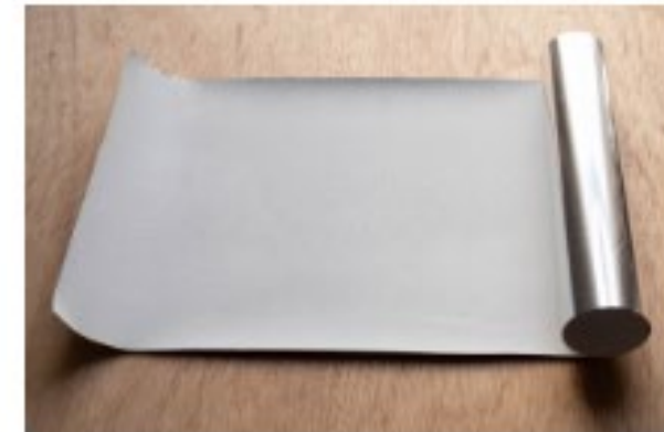
(f) Ribbon can be coiled without cracking the paint
